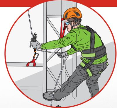
A "safety key" must be made via a knot to avoid possible handling errors.
